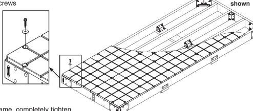
Once Dock Top is secured to frame, completely tighten all hex bolts from previous step. Then slightly loosen these
